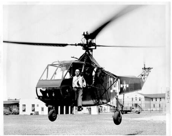
One of the early helicopter designs—the Sikorsky R4 designated the HNS-1 in US Coast Guard Service [CG 39040].
